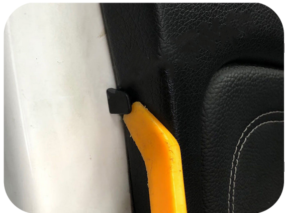
Pry up the side latch with a plastic pry tool
