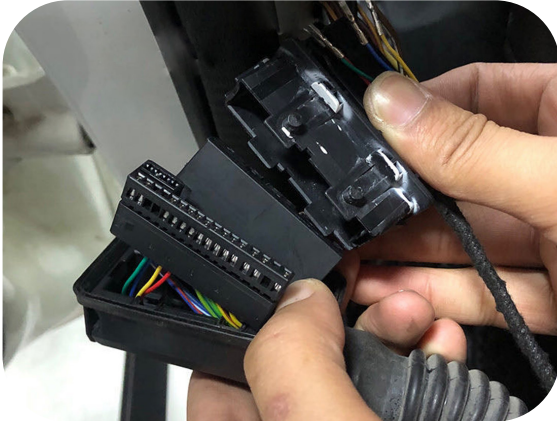
Rear door Ambient light B threading (just insert the wire by matching the colors)
