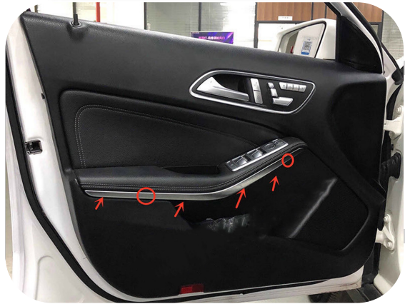
Remove the electroplated parts of the door and remove the T30 door screws
